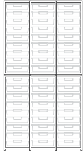
Wall Unit, 60 Module Dimensions: W 42 5/8 x H 83" x D 17"
